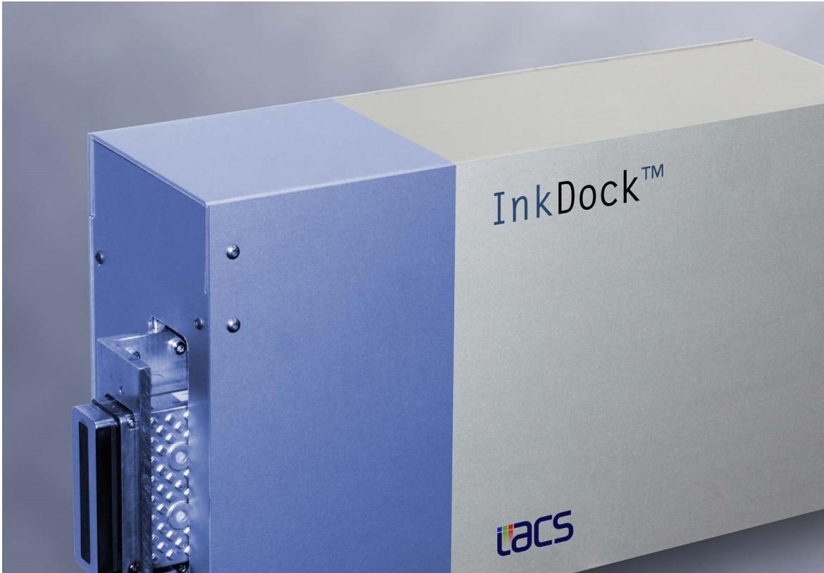
InkDock™ from IACS is a highly compact and versatile ink supply system for industrial inkjet print heads that have reflow or fluid recirculation architecture. Recent inkjet heads use recirculation to eliminate the build-up of air bubbles and pigment sediment around nozzle openings, vastly improving their reliability and minimising production down-time. Reliable jetting is particularly important in single-pass printing.
